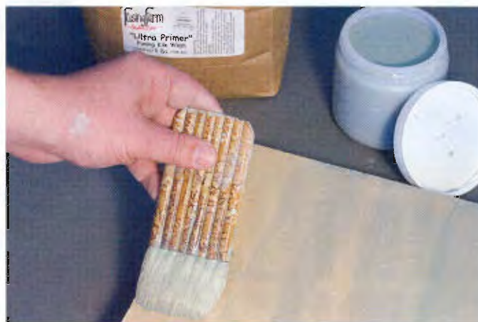
Preparing shelf with Fusing Farm Ultra Primer
